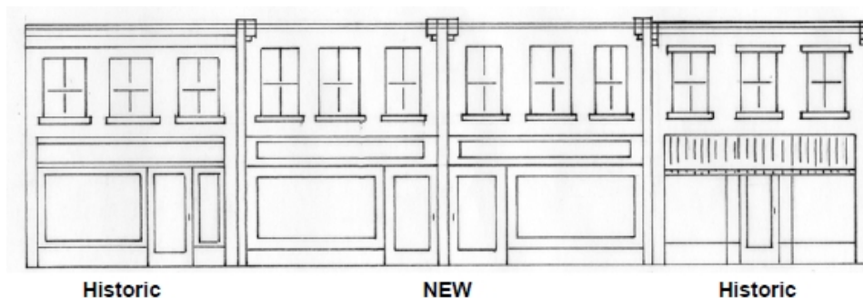
Figure 4: Appropriate New Construction - Main St.
