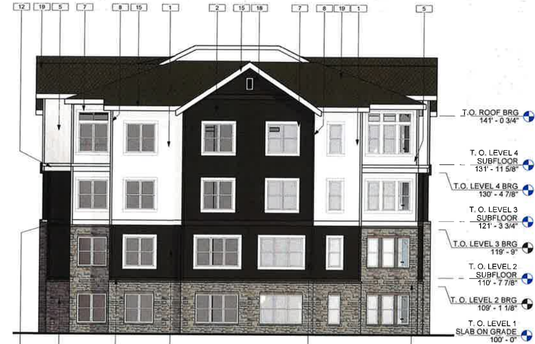
2 BUILDING A - SIDE B ELEVATION 1/8" = 1'-0"
