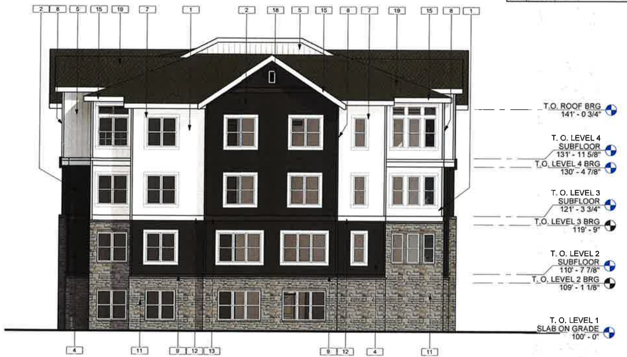
2 BUILDING B - SIDE B ELEVATION 1/8" = 1'-0"
