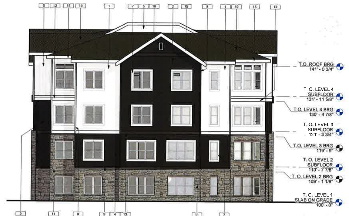
1 BUILDING A - SIDE A ELEVATION 1/8" = 1'-0"
