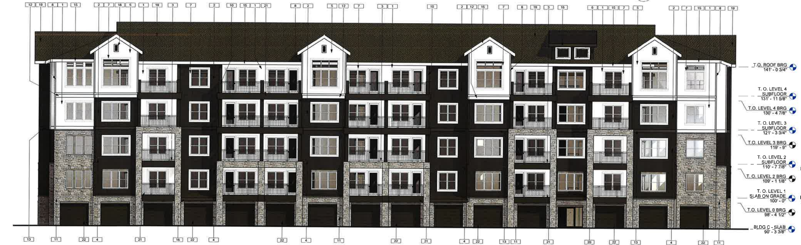
1 BUILDING C - FRONT ELEVATION 1/8" = 1'-0"
