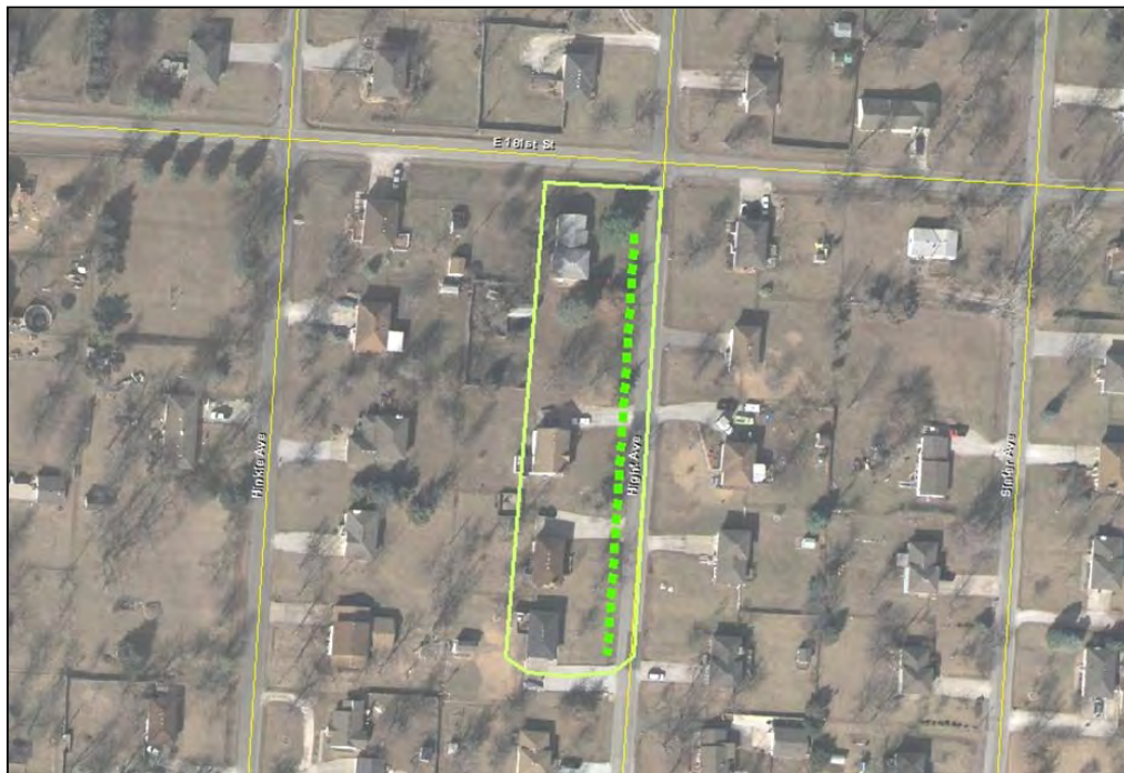
The site is typical for the area and consists of approximately 1/3 acre residential lots. Roadside ditches and driveway culverts are used to convey stormwater. It appears that the majority of the ditches in this area have not been modified since initial construction. The existing right-of-way on Hight Street is approximately 50 feet wide. For the case study it was assumed a 1.25 foot deep trapezoidal swale with a 5 foot flat bottom and 4:1 side slopes will be constructed and vegetated. A cross section illustration can be seen in the following figure.
