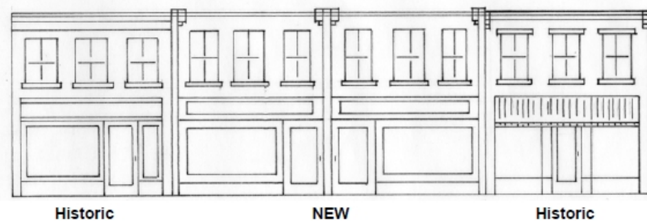
Figure 4: Appropriate New Construction - Main St.
